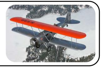
Since I last featured some pictures of David's Boeing 40C the build has progressed and is now nearing completion. The model is 1/5th scale, has a wingspan of 2.8m, and will be powered by an OS 200FS four stroke engine.
