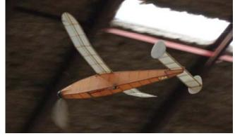
Jim Fullarton's replica of his own design Wakefield from 1949 is fitted with a single leg retracting undercarriage.
