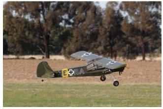
Bob Hulett is a Twin Cities member and brought this Storch for his first scale competition. The Storch is a 2.4m wingspan Austar ARF powered by a 26cc petrol engine and weighs 6.7kg.
