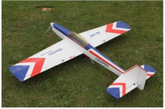
Cliff's other model was a "Calypso" produced in 1983 by Model Tech. Model is powered by an OS 61 Hanno Special.
