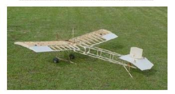
Ken's flying model of the Robbins and Porter aircraft was built from a three view prepared by the Albury Historical Society and based on recorded dimensions and photographs of the actual aircraft, taken in 1913.
