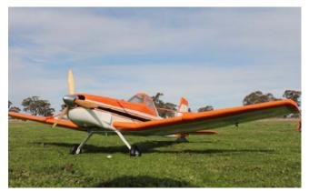
Glen Weeks' Cessna 188 is an ARF by Austar. At 2.8m wingspan it weighs 11kg and is powered by an OS Super Gemini 300 twin.
