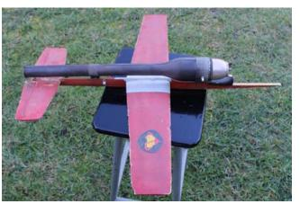
David's speed model from the early 90's, powered by an OS pulse jet and missing only the fuel tank.
