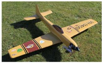
Norm Morrish was flying a model which was "state of the art" in 1972. The model, a "Northerner" was designed and built by the late John McGrane and was a highly successful aerobatic event winner. Norm built a new fuselage to replace the oil soaked original but the rest of the model is as built in 1972. Powered by a Webra Speed 61 two stroke it flew the Classic schedule very well in Norm's capable hands.
