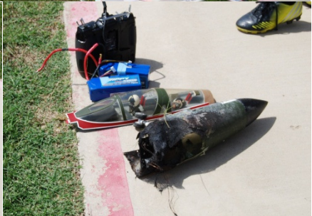
Above three photos show the remains of the F-4E after an in-flight ESC fire. YUCK!
