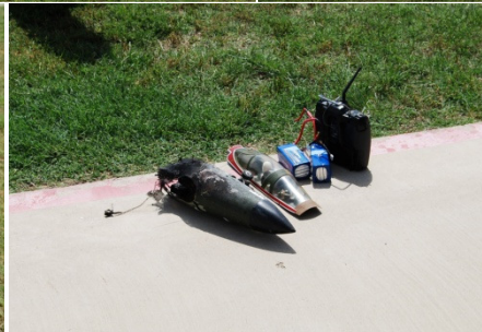
Above three photos show the remains of the F-4E after an in-flight ESC fire. YUCK!
